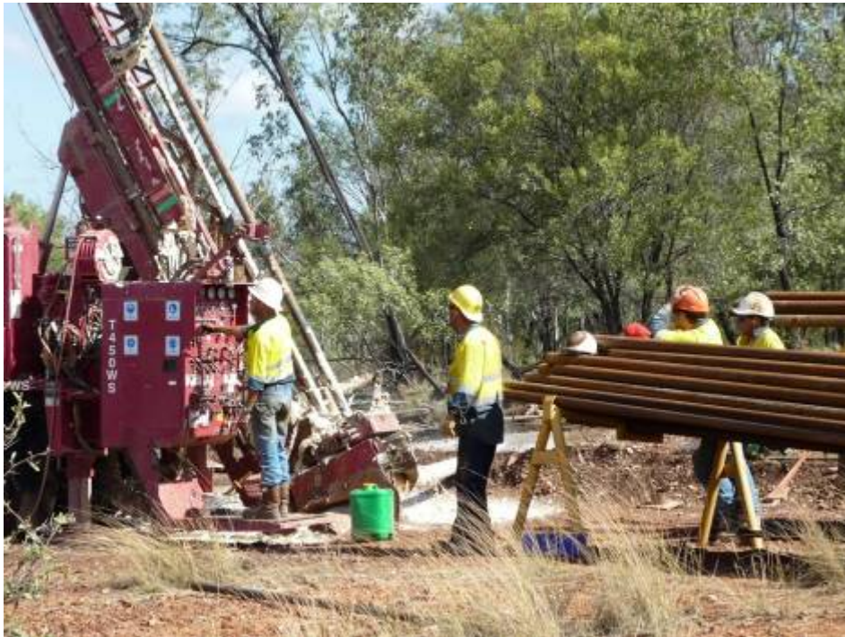
RC drilling at Anthony, November 2009
