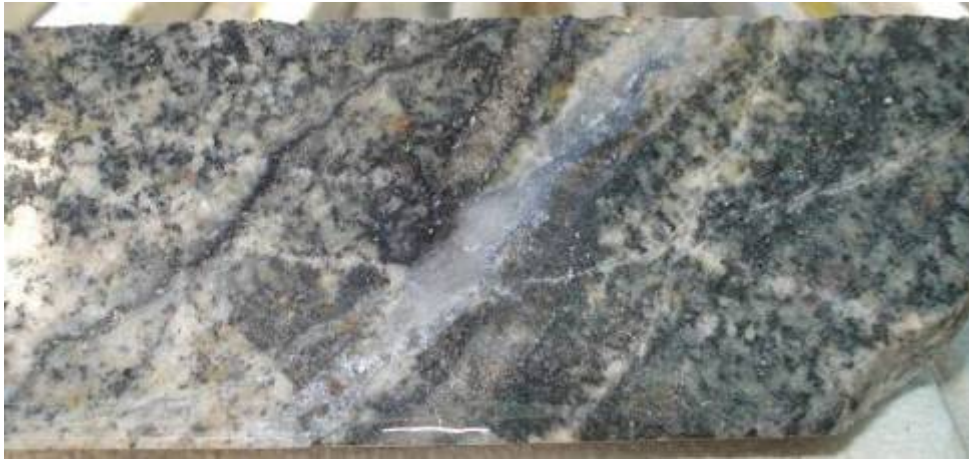
Anthony prospect - sawn drill core showing quartz-Mo veins in altered granite. Molybdenite [MoS 2 ] is the silvery-grey mineral. Hole RCD09-19, depth 207.3m
